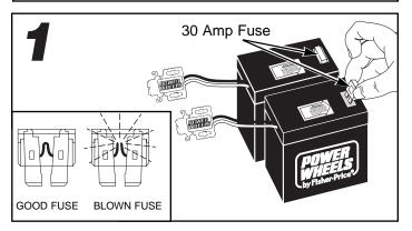
• If you are charging the batteries for the first time, insert a 30 amp fuse into each battery before charging.
